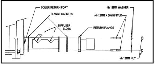
Figure 15. Return Diffuser Installation
